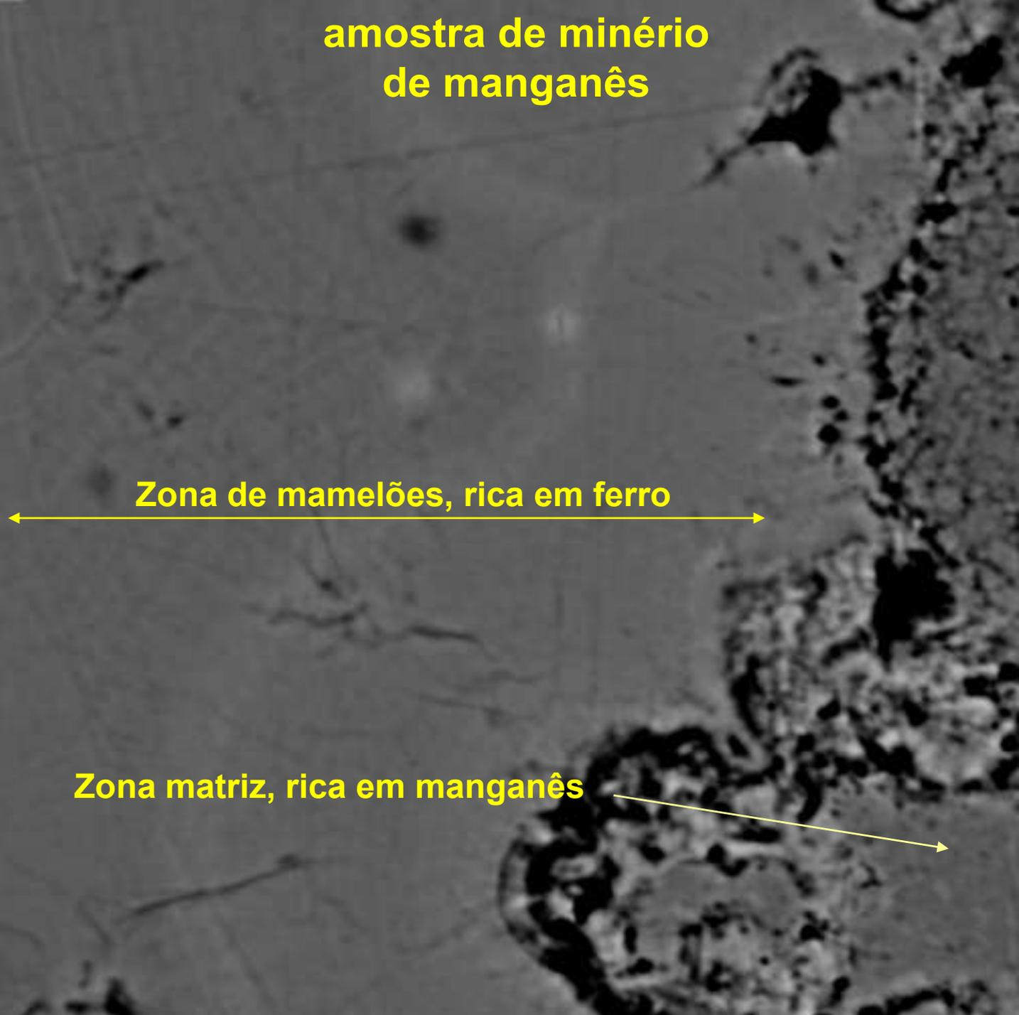
A grayscale backscattered electron (BSE) image of a manganese ore sample. The image shows a complex microstructure with a matrix and a zone of nodules. A yellow double-headed arrow points to a horizontal band in the upper-middle section, labeled 'Zona de mamelões, rica em ferro'. Another yellow arrow points to a darker, more textured region on the right side, labeled 'Zona matriz, rica em manganês'. The overall appearance is granular with some darker, more irregular shapes.
