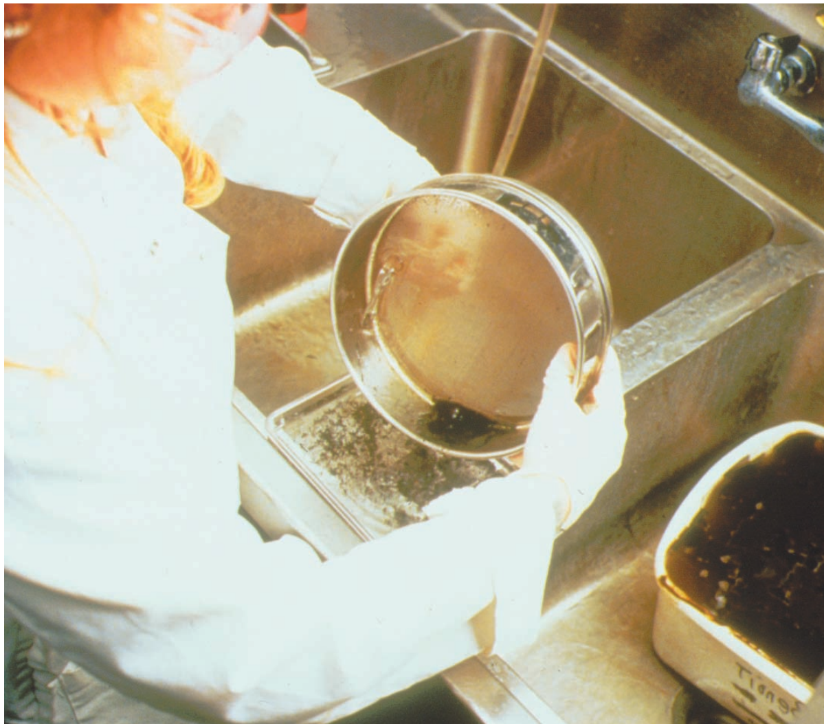
Sieving a sediment sample for toxicity testing
