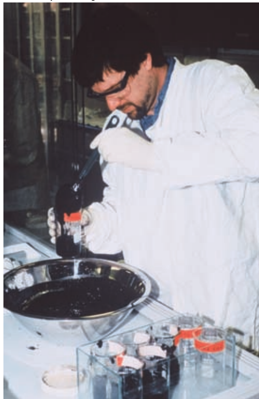
Subsampling sediment for toxicity testing
